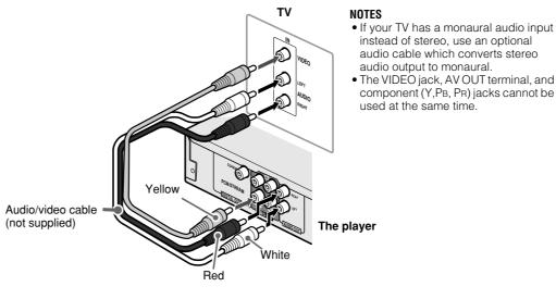
The VIDEO jack, AV OUT terminal, and component (Y,PB, PR) jacks cannot be used at the same time
